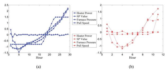
Figure 5. Selected standardized process variables in a CZ process (a) a conforming batch and (b) a batch containing polycrystalline defects.
